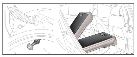
When returning the seat back to the upright position ensure that the seat belts are routed correctly and are not trapped by the seat back. Press the seat back firmly and check that it is locked securely into place.
