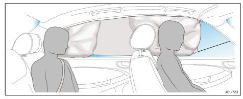
When the curtain airbag inflates upon a vehicle side impact, it breaks through the headlining and deploys downwards, giving head protection to front and rear seat occupants.
