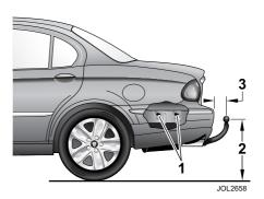
The rear longitudinal members are factory pre-marked (1) for drilling for tow-bar mountings. There are two tow-bar mounting points on either side of Saloon models, and three mounting points on either side of Estate models.
