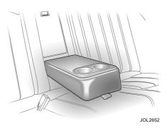
Pull the loop on the rear centre armrest to lower. If not required, raise the armrest to its upright position and push firmly into place. Ensure that the armrest is raised when lowering the seat back to increase the luggage compartment area.
