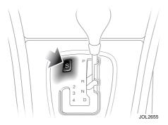
The switch marked 'S' on the 'J'-gate surround enables the driver to select either normal 'N' or sport 'S' modes.
