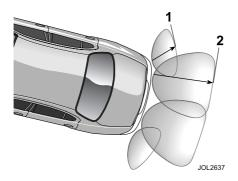
When reverse gear is selected and the ignition is on, rear parking assist provides an audible warning when reversing the vehicle if obstacles are detected within range of the rear of the vehicle, as shown in the illustration above.
