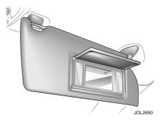
Adjustable sun visors can be swung downwards or unclipped and swung sideways to reduce sun glare.
