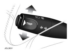
The direction indicators operate when the ignition is in position 'II'. To indicate for a right or left turn, move the column left stalk switch up or down respectively. The switch will cancel when the turn is completed.
