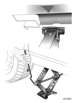
There are four jacking points, two each side of the vehicle on the underside of the floor. These provide positive location for the jack.
