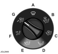
The rotary control has seven main air distribution positions but the air distribution changes continuously between positions as the knob is rotated. The control knob may therefore be set at any point for optimum comfort.
