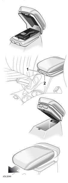
The sliding armrest is hinged at the rear and has two release buttons located on the front of the armrest.
