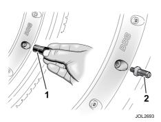
These wheels have a slotted valve cover on the wheel face. A pouch containing a special tool and a valve adaptor, for use with these wheels, is stowed in the glove compartment.
