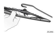
Move the wiper arm away from the windscreen, squeeze the retaining clip and withdraw the wiper blade from the arm. After fitting the new blade, check that it is held firmly in position. Reposition the wiper arm and blade onto the screen.
