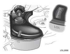
The coolant level must only be checked when the engine is COLD.
