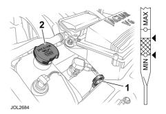
Remove the dipstick (1) and wipe clean with a non-fluffy cloth. Replace fully, then withdraw the dipstick. If the oil level is above the minimum mark on the dipstick then no additional oil is required.
