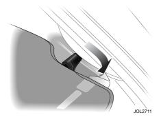
The luggage cover can be extended to hide the contents of the luggage compartment. The cover retracts into the housing when not required.
