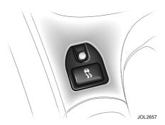
All 2.0 litre petrol and diesel-engine vehicles are fitted with traction control as standard. The system will intervene to prevent wheel spin, by automatically reducing the power output from the engine and applying braking to individual wheels.
