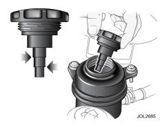
Caution: It is imperative that the power steering system does not become contaminated in any way. Always dispense fluid from a fresh sealed container and clean the area around the reservoir neck both before and after replenishment. Never return drained fluid to the system.
