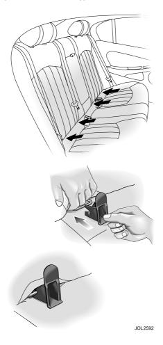
Only the Britax Roemer 'Duo Plus' ISOFIX restraint is approved by Jaguar for use with this system. An ISOFIX anchorage kit must be fitted to your vehicle before the ISOFIX seat can be installed.
