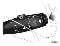
Push the button on the end of the switch to obtain the wash/wipe programme.
