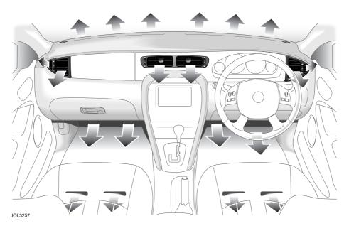
The illustration shows the location of the air vents within the vehicle.
