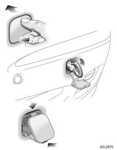
The front towing point is located behind a square cover on the face of the bumper on the left-hand side of the vehicle. To access the towing point, push the top of the tow point cover inwards and upwards, which will cause the cover to pop out of place. Lift the cover from the access hole. The tow point cover is attached to the vehicle by a retaining strap.
