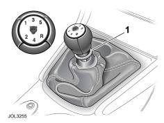
A diagram of the gearshift pattern is set in the top of the lever knob.
