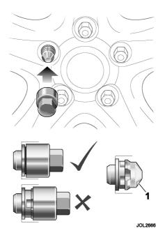
Where Jaguar locking wheel nuts are fitted (one on each wheel), they can only be removed using the correct key socket.
