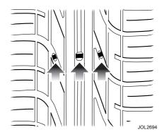
It should be noted that the properties of many tyres alter progressively with wear. In particular the 'wet grip' and aquaplaning resistance are gradually but substantially reduced. Extra care and speed restriction should therefore be exercised on wet roads as the effective tread depth diminishes.
