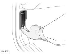
Pull the release lever located below the fascia on the left-hand side of the vehicle, see page 180.
