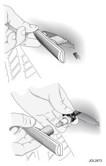
Remove the light unit by pushing the lens towards the front of the vehicle to compress the spring clip and then pull the rear outwards to remove the complete unit.
