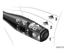
Estate models are fitted with a rear screen wash/wipe. This is operated by the right-hand column stalk and only operates with the ignition in position 'II'.
