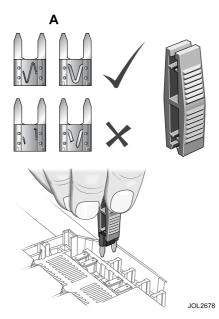
Although there are several types of fuse used in the vehicle, only 'mini-fuses' (**A**) can be changed by the owner.
