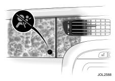
The front passenger seat is equipped with a sensor that determines if the seat is occupied by measuring the weight on the cushion. This information is used to change the passenger airbag deployment status.
