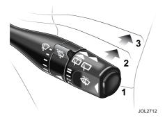
Estate models are fitted with a rear screen wash/wipe. This is operated by the right-hand column stalk and only operates with the ignition in position 'II'.
