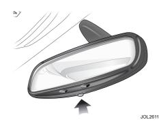
Push the switch in and the electrochromic rear view mirror darkens automatically to prevent glare from a following vehicle's headlights. The mirror clears when light levels return to normal. The mirror also clears when reverse gear is selected.
