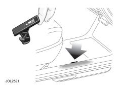
Pull the fuel filler flap release. This is located on the floor, outboard of the driver's seat, see page 134.
