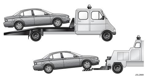
When the vehicle is being transported on a trailer or vehicle flat bed transporter, the handbrake must be applied, the wheels chocked and:
