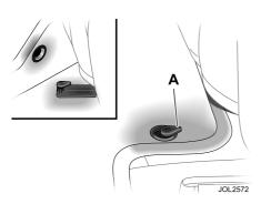
Ensure that the driver's floor mat is correctly positioned and secured under the tongues on the retention posts (**A**, only one post shown), so that the mat does not interfere with the operation of the accelerator, clutch or brake pedals. In particular, check the position of the mat
