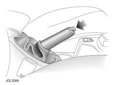
The handbrake lever, which applies the parking brakes, is mounted on the centre console beside the driver's seat.
