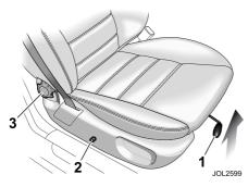
Forward and rearward: Each front seat can be adjusted forward and rearward by lifting the locking bar (1), situated below the front of the seat cushion and sliding the seat to the required position.
