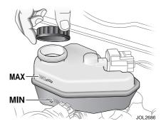
The manual transmission clutch fluid is shared with the brake fluid in a common reservoir
