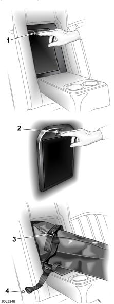
A two-door hatch is fitted to the rear seat of some Saloon models. When open, this gives a space for skis or similar objects to be stowed in the vehicle. Both doors have a single catch.
