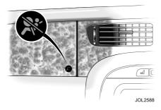
The front passenger seat is equipped with an occupancy sensor. The sensor measures the weight on the cushion and changes the passenger airbag (5, see page 53) deployment status.
