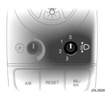
The headlight levelling switch operates when the headlights are switched ON. Push and release the knob to extend it for ease of operation. Push the knob again to place it in the stowed position.
