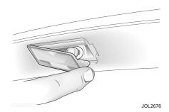
Push the lens clip sideways and remove the lens from the vehicle.
