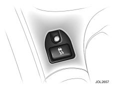
Dynamic stability control is operational whenever the engine is running, unless it has been switched off. If the system is operating, the warning light in the instrument cluster will flash.
