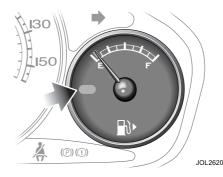
An amber lozenge in the fuel gauge illuminates when the remaining fuel has fallen to approximately 8 litres (1.75 gallons) including the reserve.
