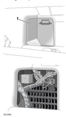
To locate the fuse box, open the glove compartment and pull out the panel (1). The fuse box is visible through the aperture.
