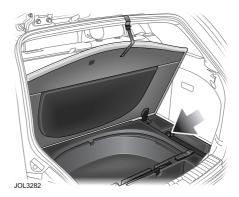
A 12-volt accessory socket is provided in the underfloor storage tray. The socket must only be used to power accessories that are temporarily connected to the vehicle.
