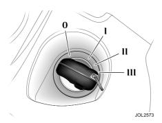
The ignition switch, on the right-hand side of the steering column, has four key positions:
