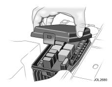
The fuse box is located in the engine compartment on the left-hand side adjacent to the battery.
