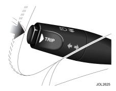
Press the TRIP button to cycle through: TRIP - ODOMETER - MESSAGES - CLOCK (where available).
