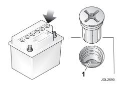
**Note:** In normal climates this must be carried out at least once a year. In hot weather/climates the electrolyte level must be checked at least every three months.
