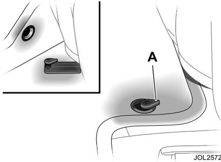
Ensure that the driver's floor mat is correctly positioned and secured under the tongues on the retention posts (A, only one post shown), so that the mat does not interfere with the operation of the accelerator, clutch or brake pedals.
