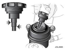
Caution: It is imperative that the power steering system does not become contaminated in any way. Always dispense fluid from a fresh sealed container and clean the area around the reservoir neck both before and after replenishment. Never return drained fluid to the system.
