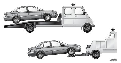
When the vehicle is being transported on a trailer or vehicle flat bed transporter, the handbrake must be applied, the wheels chocked and:
