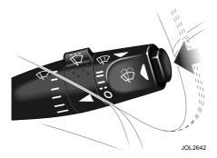
Push the button on the end of the switch to obtain the wash/wipe programme.
