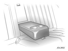
Pull the loop on the rear centre armrest to lower. If not required, raise the armrest to its upright position and push firmly into place. Ensure that the armrest is raised when lowering the seat back to increase the luggage compartment area.
