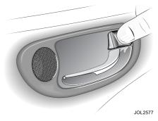
To centrally lock all doors, press the lock lever on the driver's or front passenger's door.
