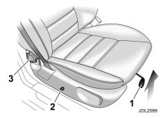
**Forward and rearward:** Each front seat can be adjusted forward and rearward by lifting the locking bar (1), situated below the front of the seat cushion and sliding the seat to the required position. After releasing the locking bar, slight additional seat movement may be necessary to engage the locking mechanism.
