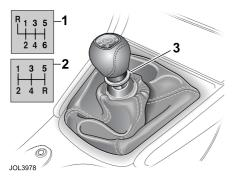
A diagram of the gearshift pattern, either 6 speed (1) or 5 speed (2) is set in the top of the lever knob.
