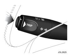
Press the TRIP button to cycle through: TRIP - ODOMETER - MESSAGES -CLOCK (where available).
