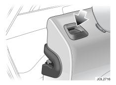
There is a red indicator to the rear of each release catch, which is only visible when the seat is unlatched.
