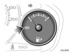
An amber lozenge in the fuel gauge illuminates when the remaining fuel has fallen to approximately 8 litres (1.75 gallons) including the reserve.
