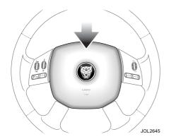
The dual tone horn is operated by pressing the centre pad on the steering wheel.
