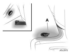
Ensure that the driver's floor mat is correctly positioned and secured under the tongues on the retention posts (**A**, only one post shown), so that the mat does not interfere with the operation of the accelerator, clutch or brake pedals.
