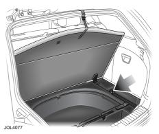
A 12-volt accessory socket is provided in the underfloor storage tray. The socket must only be used to power accessories that are temporarily connected to the vehicle.
