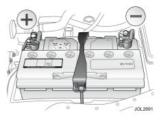
Open the bonnet and unclip the battery box cover. Remove the positive terminal cover.
