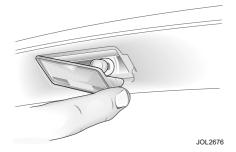
Push the lens clip sideways and remove the lens from the vehicle.
