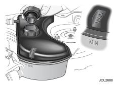
The coolant level must only be checked when the engine is COLD.
