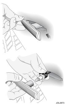
Remove the light unit by pushing the lens towards the front of the vehicle to compress the spring clip and then pull the rear outwards to remove the complete unit.
