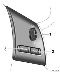
The cruise (speed) control system (where fitted) can be used by the driver to maintain a selected vehicle speed above 28 km/h (18 mph) for 2.5- and 3.0-litre vehicles, and 40 km/h (25 mph) for 2.0-litre petrol and diesel vehicles, without the driver having to use the accelerator.
