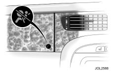
The front passenger seat is equipped with a sensor that determines if the seat is occupied by measuring the weight on the cushion. This information is used to change the passenger airbag deployment status.
