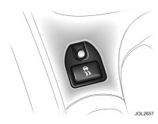
2.0 litre petrol and all diesel-engine vehicles are fitted with traction control as standard. The system will intervene to prevent wheel spin, by automatically reducing the power output from the engine and applying braking to individual wheels.
