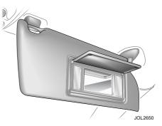
Adjustable sun visors can be swung downwards or unclipped and swung sideways to reduce sun glare.
