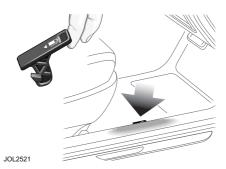
Pull the fuel filler flap release. This is located on the floor, outboard of the driver's seat, see page 127.
