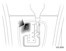
The switch marked **S** on the J-gate surround enables the driver to select either normal **N** or sport **S** modes.
