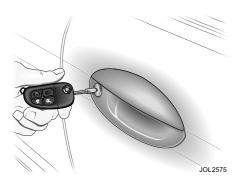
All doors can be locked and unlocked either remotely using the key transmitter buttons, or by using the integrated key.
