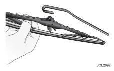
Move the wiper arm away from the windscreen, squeeze the retaining clip and withdraw the wiper blade from the arm. After fitting the new blade, check that it is held firmly in position. Reposition the wiper arm and blade onto the screen.
