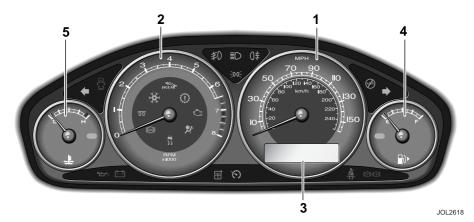
None of the instruments will show correct indications until the ignition is switched ON (position **II**).
