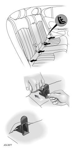
Only the Britax Roemer Duo Plus ISOFIX restraint is approved by Jaguar for use with this system. An ISOFIX anchorage kit must be fitted to your vehicle before the ISOFIX seat can be installed. These brackets must be supplied and fitted by your Jaguar Dealer/Authorised Repairer. The ISOFIX anchorage kit and the ISOFIX seat cannot be installed in Estate models.
