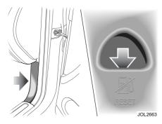
In the event of an accident, an inertia switch will trip, isolating the fuel supply. Once the switch has tripped it must be reset before attempting to restart the engine.
