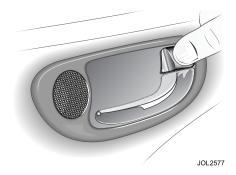
To centrally lock all doors, press the lock lever on the driver's or front passenger's door.
