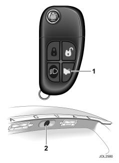
If the vehicle alarm system is armed and the luggage compartment is opened using the key transmitter the alarm will not sound. The system will be rearmed when the lid is closed, provided the vehicle has not been disarmed.
