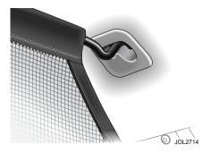
A luggage load net is fitted to some luggage cover housings. This can reduce the risk of luggage being thrown forward in the event of an accident, or under heavy braking. The load net can be retracted into the housing when not required.
