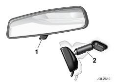
Interior mirrors are either manual dip or electrochromic.
