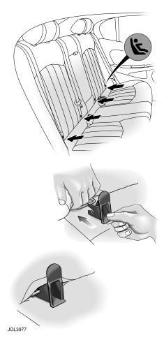
Only the Britax Roemer Duo Plus ISOFIX restraint is approved by Jaguar for use with this system. An ISOFIX anchorage kit must be fitted to your vehicle before the ISOFIX seat can be installed. These brackets must be supplied and fitted by your Jaguar Dealer/Authorised Repairer. The ISOFIX anchorage kit and the ISOFIX seat cannot be installed in Estate models.
