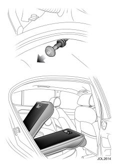
**Saloon:** Release handles for each seat back are in the luggage compartment under the parcel shelf. Pull the handle to release the seat back.
