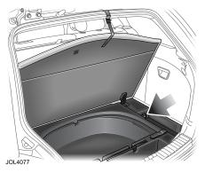
There is an underfloor storage tray located below the floor panel. Lift the floor panel (there is a handle on the rear edge) to access the storage tray.
