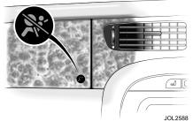
The airbag indicator light (occupancy sensing) is located on the passenger fascia.
