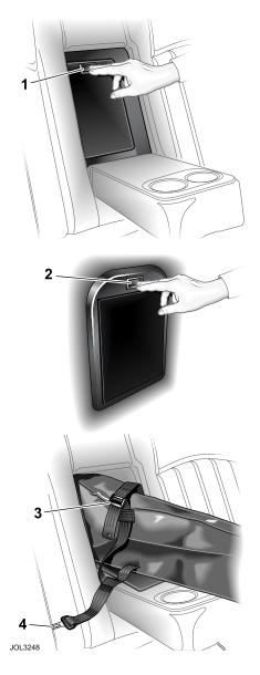
A two-door hatch is fitted to the rear seat of some Saloon models. When open, this gives a space for skis or similar objects to be stowed in the vehicle. Both doors have a single catch.
