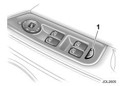
Front windows on all models are electrically operated. Depending on the model, rear windows can be either manually or electrically operated.
