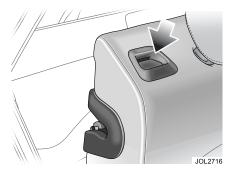
**Estate:** Release catches are located on the top of each seat back. Press the catch to release the seat back.
