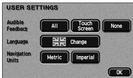
After touching the **User Settings** button, the screen displays the buttons for the selection of audible feedback, language, and units of measurement.
