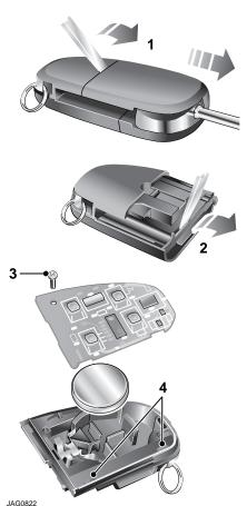
When the battery needs renewal there will be a significant decrease in the effective range of the key transmitter. To renew the battery, follow the procedure below:
