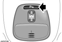
When both front and rear parking assist are fitted, a switch is located in the overhead console.
