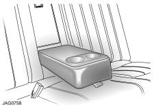
Pull the loop on the rear centre armrest to lower. If not required, raise the armrest to its upright position and push firmly into place. Ensure that the armrest is raised when lowering the seat back to increase the luggage compartment area, see *'CUPHOLDERS'*, page 126 for further information related to this feature.
